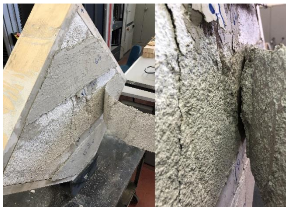
Fig. 13. Collapse of the reinforcement strip
