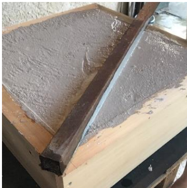
Fig. 6. Creation of the upper layer of mortar.
