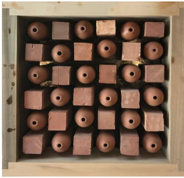
Fig. 4. Arrangement of bricks and NFTs in the timber frame.
