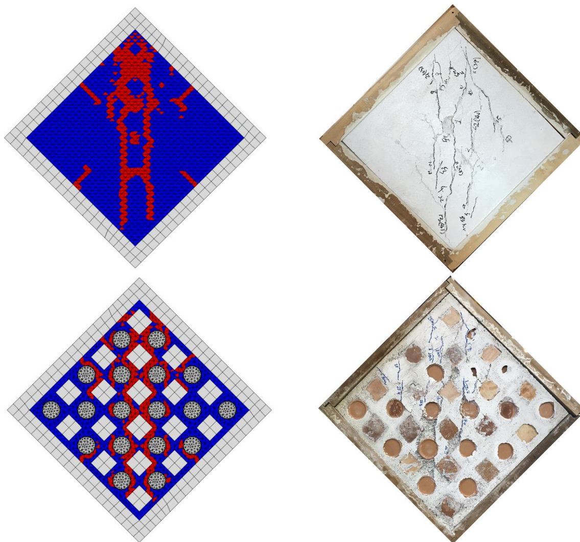
Figure 16. Comparison of cracks development in in the back and front side of numerical model and experimental specimen wall.
